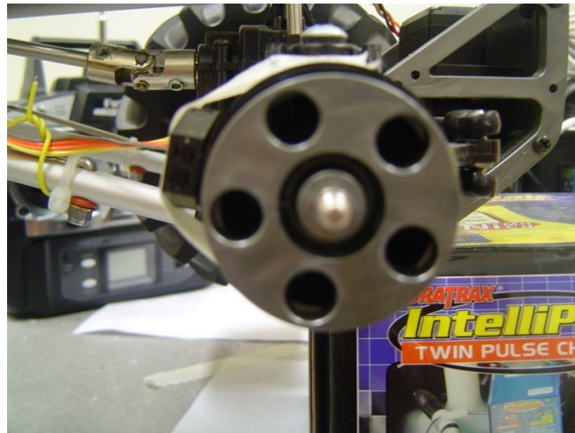
Figure 5 Image of Opto-Reflective Switch mounted inside wheel hub
